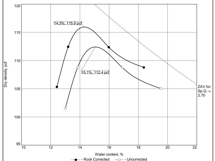
Test specification: ASTM D 698-12 Method C Standard ASTM D4718-15 Oversize Corr. Applied to Each Test Point
